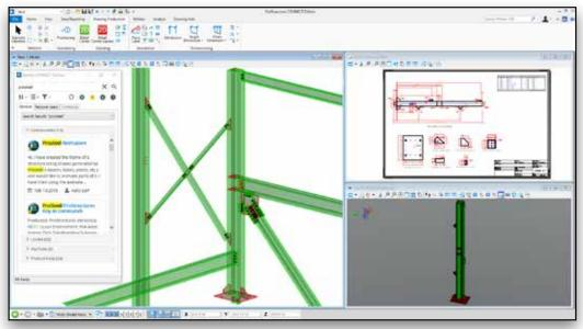
ProSteel automatically updates all drawings based on changes to the 3D model, and CONNECT Advisor has been integrated into ProSteel as a unified interface to various Bentley content.
