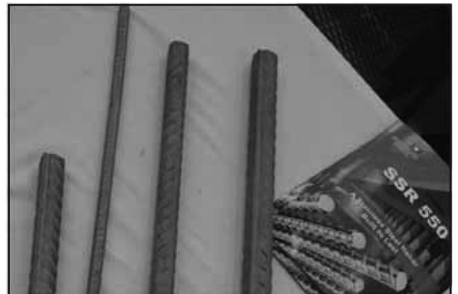
Fig. 12 Ferritic Stainless Steel reinforcement bars
